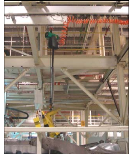
Location: Shanghai General Motors Application: JDN Air Hoist mini 125 operating in a paint shop. Sender: Gary Lee, Shanghai
